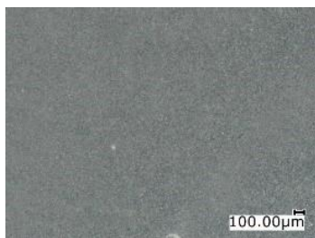
FIGURE 1. Microscopic photo of ZnO layer obtained by droplet deposition method using a slurry obtained from zinc acetate and oleic acid in a molar ratio of 1 to 2
